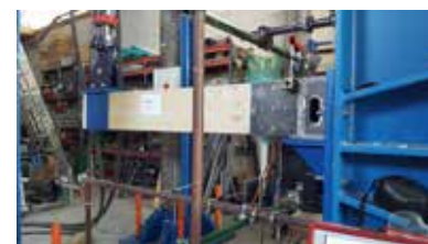
Test spoja les-jeklo – projekt Tigr4Smart Test of timber-to-steel joint – project Tigr4Smart
