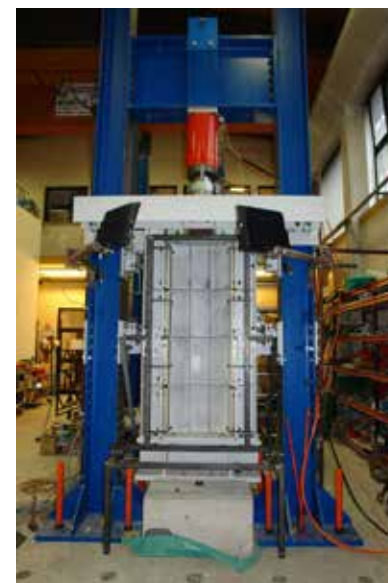
Test ojačene ukrivljene jeklene pločevine v tlaku – projekt RFCS OUTBURST Test of curved stiffened steel panel – project RFCS OUTBURST
