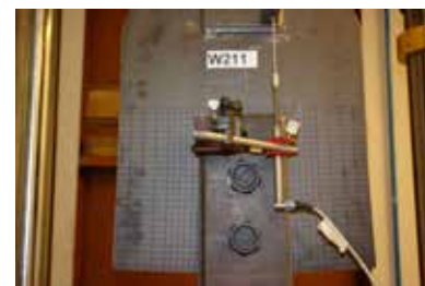
Test polno nosilnega spoja med stebrom in prečko Test of a full strength beam-to-column joint
