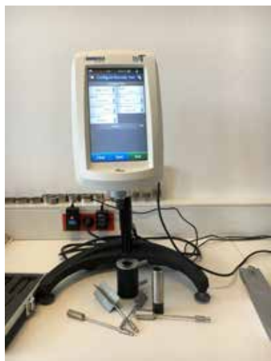
Rheometer, s katerim smo na Katedri za mehaniko tal vpeljali meritve reoloških lastnosti sedimentov iz vodnih okolij, zalivnih mas in drugih sorodnih materialov Rheometer introduced at the Chair of Soil Mechanics for the investigations of rheological properties of sediments from water environments, injection masses and other similar materials
